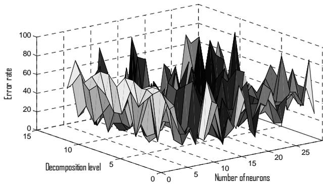
Figure 8: Error rate of the ANN system vs. decomposition level and number of neuron.
