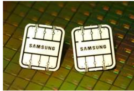
Figure 2.11: Solid-state micro-controller from Samsung (S3CC9EF) with 256 kB storage and ISO 7816 compliance (Samsung website).
